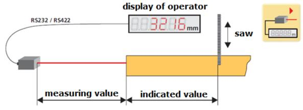
Additionally, you can connect the measuring device through a 15 pin D-sub plug. Alternatively, you can run a cable directly into the device through a cable gland and connect it to the internal terminals. Optionally the connection to a Profibus-Master is also possible.
